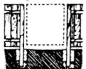
two gates posts to ensure the gate can swing freely. After the gate has been constructed properly for the space desired, attach the hinges and gate latch. If you desire a stop, nail a piece of fencing material to the latch post.
